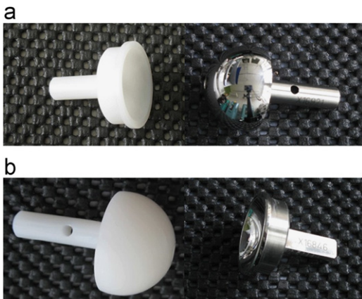
Fig. 1. (a) Test samples—pairing 1: PE-Inlay versus CoCr-Glenosphere. (b) Test samples—pairing 2: PE-Glenosphere versus CoCr-Inlay.
